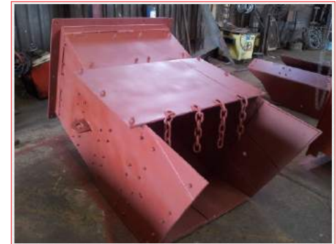
Fabricated Ore-pass Chute
